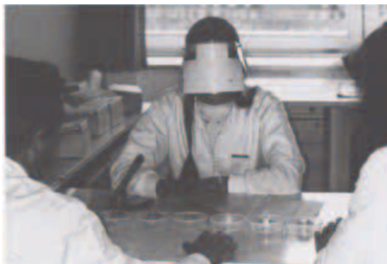
Figure 2 Testing of initial acceptance. The test subjects were blindfolded, presented eight appliances in pairs (altogether 56 pairs for each subject) and requested each time to state their preference as to which of the two was more comfortable to wear.
